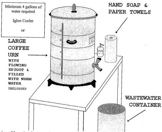
If your stand is without a hot and cold running (pressurized) water supply, then use the diagram to set up an acceptable hand wash station.
